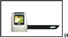
Insert the negative holder into the slot on the right side of the Virtuoso® Film Scanner as shown. Slide the negative or film inside the holder until your first photo appears on the preview screen without its edges being cut off.
