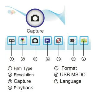
If you are in capture mode, press the "MENU" button twice to open the Main Menu. The Main Menu displays five icons that are used to access the various features of the Virtuoso® Film Scanner:
