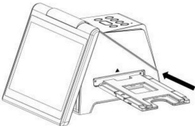
*Inserting the main holder into the device.*
