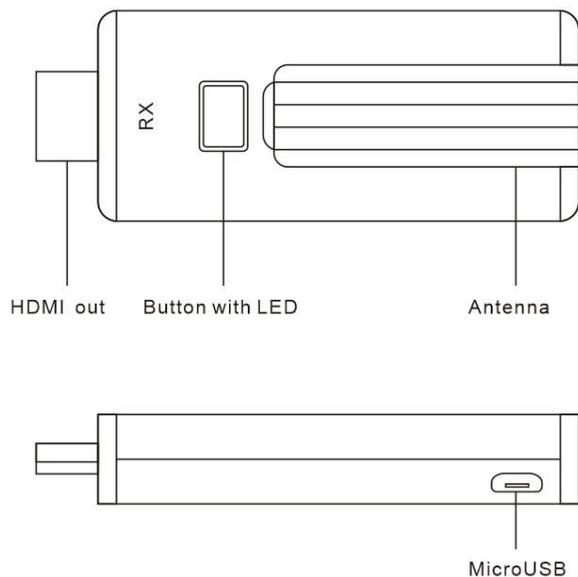
**1. HDMI OUT:** Connect to a TV or monitor. NOTE: For the receiver (RX), external power is always required. You will need to connect the USB power cable to the receiver's microUSB port to provide enough power to the receiver.
